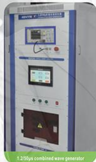
1.2/50μs combined wave generator
