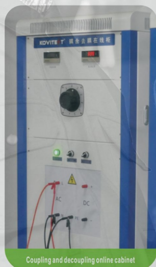
Coupling and decoupling online cabinet
