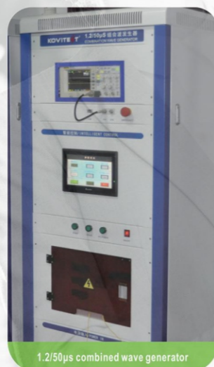
1.2/50µs combined wave generator
